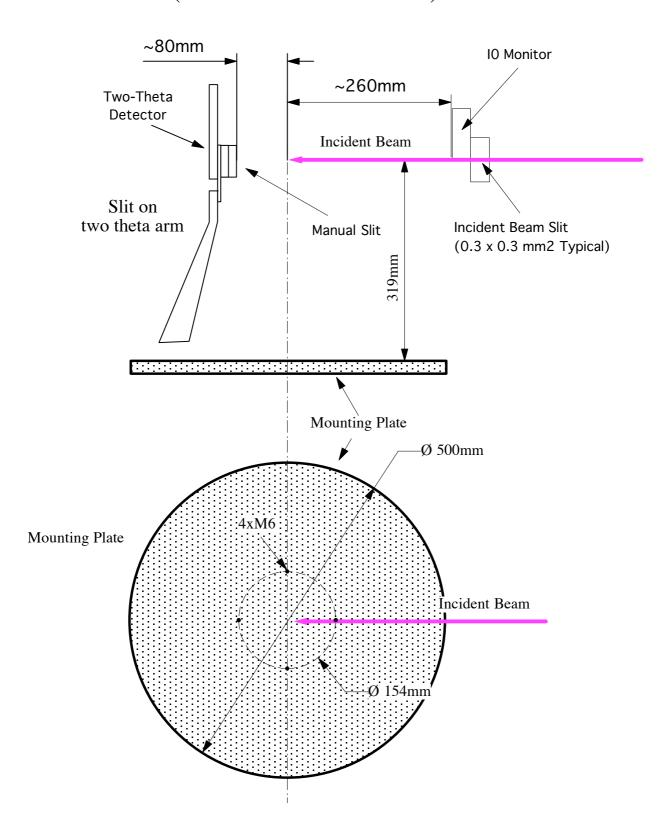
Note: The height (319 mm) can easily be adjusted +-5 mm.
